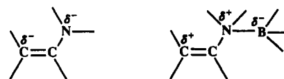
Figure 4. Reversal of the normal electronic effect of the enamine dialkylamino group due to coordination of the hydroboration reagent with nitrogen.
